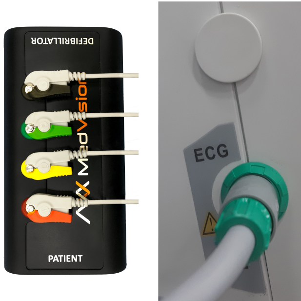
Figure 2.11 Connecting the monitor to the unit
